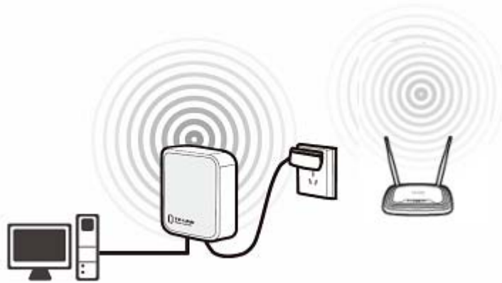
Figure 2-5 Hardware Installation of the TL-WR702N in Client Mode
