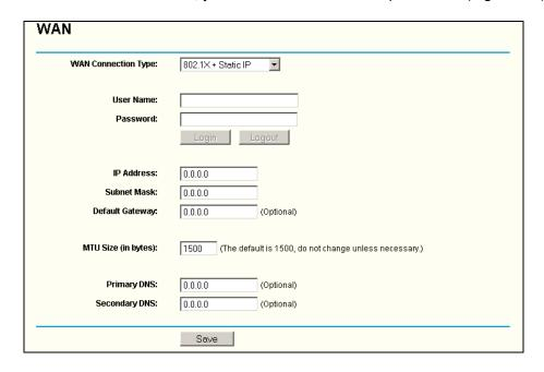
Figure 4-9 802.1X + Static IP Settings
