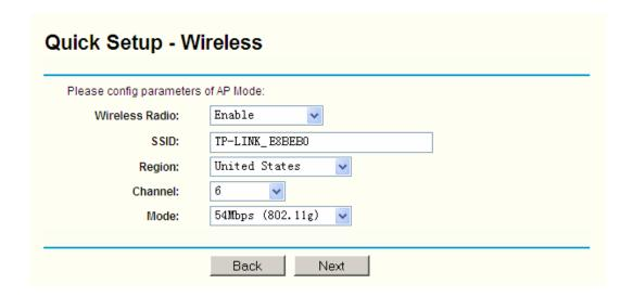
Figure 3-9 Quick Setup - Wireless settings
